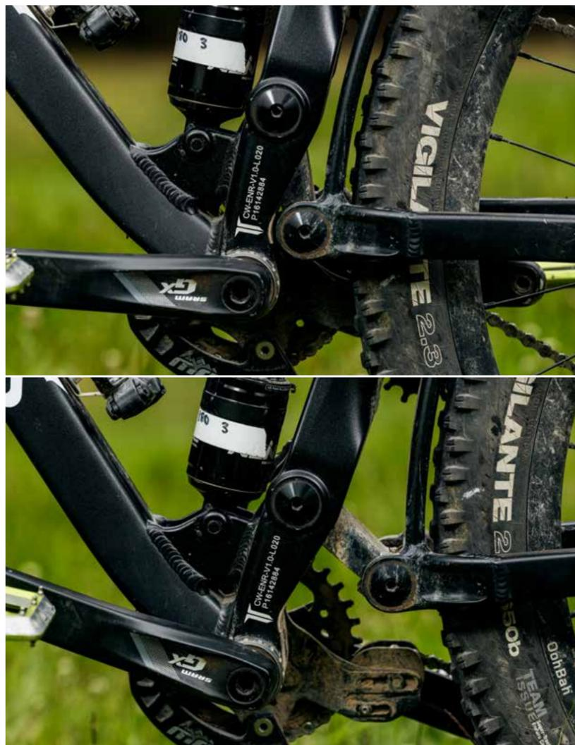
THE AMOUNT OF REARWARD TRAVEL, PART WAY THROUGH COMPRESSION, IS CLEARLY VISIBLE IN THESE TWO SHOTS IF YOU LOOK AT HOW FAR FURTHER BACK THE WHEEL IS IN COMPARISON TO THE CHAINRING IN THE SECOND PICTURE.
